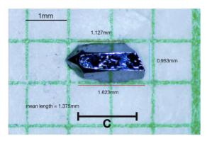
FIG. 8. Most of the magnetic measurements were done on the LaCrGe<sub>3</sub> crystal pictured. One side was lightly polished flat and parallel to the opposite face. We determined the size from pictures of the sample on mm grid paper. From these measurements we were able to estimate the demagnetization factors  $N_a$ ,  $N_b$ , and  $N_c$ .
